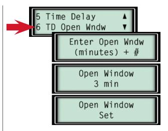
If there is an active time delay in the lock, you will have to wait through the existing time delay period before yo can change the opening window value. After you enter the new opening window value and #, the time delay countdown screen displays. When it reaches zero, you will be asked to enter the lock's master code as verification of the change and your authority to make the change.
