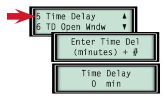
The time delay counts down from the existing delay period, then the display prompts you to confirm the master code.
