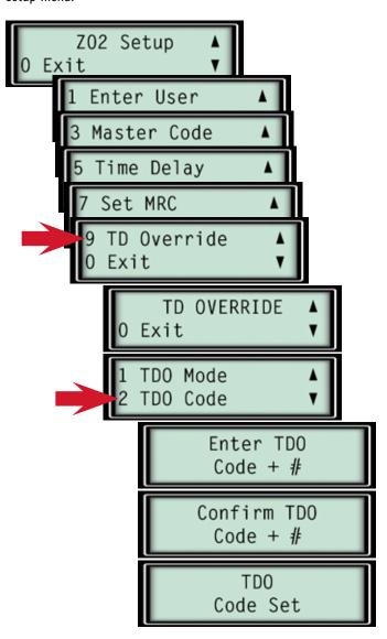
If a TDO code already exists, it can be changed by simply entering a new TDO code following this procedure.
