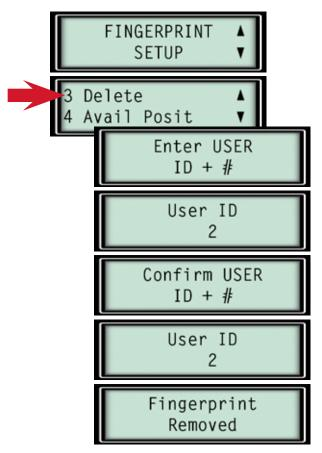
The keypad display will alert you if you attempt to delete a fingerprint from an empty PIN position, just as it would alert you if you tried to enroll a fingerprint in position that was already in use. The keypad display makes setting up and maintaining your lock parameters and data very intuitive.
