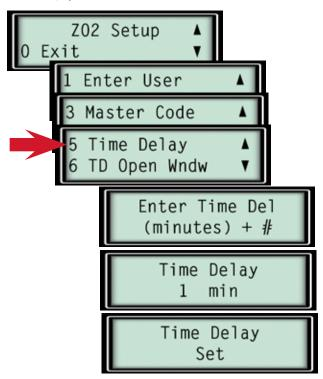
Simply enter a time value when prompted by the display to do so. The value can be anything from 1 to 9 minutes for a model 6120 lock, and anything from 1 to 99 minutes for a model 6123 or  $Z^{02}$ . The example above shows a value of 1 minute programmed into the lock.
