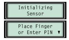
Press \* to get the lock to prompt you for the setup code, which in this case will be the #2 PIN code (supervisor code).
