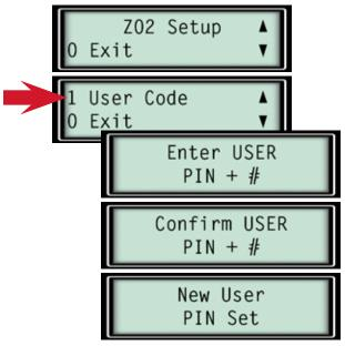
User codes can be set, changed, or deleted by the holder of either the master code or the supervisor code. They also have the ability to change themselves, as long as the lock model is either a 6123 or  $\mathsf{Z}^{02}$ .
