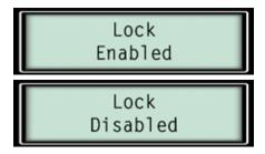
When the lock is enabled, it can be unlocked by any of the user codes in PIN positions 3 through 7. The keypad can be set for operation by fingerprint, PIN, or fingerprint <u>and</u> PIN in supervisor/subordinate mode.
